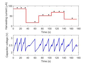
Figure 2: Capacitor voltage behavior when executing different tasks considering different energy harvesting rates during the experimental time
